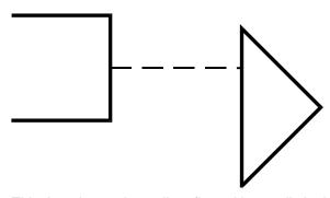
This time the ray is totally reflected internally in the prism twice and returns on a path that is parallel to its original one but reversed in direction.
