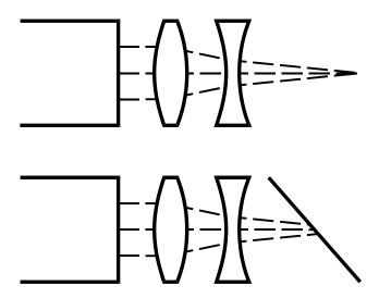
Place a plane mirror across the rays at an angle and record the paths of the reflected rays.
