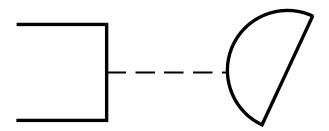
• Is the ray at this flat face refracted towards or away from the normal at the point of incidence? Again rotate the block about the centre point of the flat side and observe and record the emergent ray at the new position.
