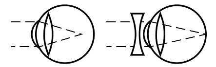
They are also used to increase the focal length of converging lenses.
