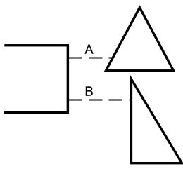
Place prisms with 60° and 30° angles as shown in the diagram, and trace the path of the emergent rays. Rearrange the prisms as shown in the diagram below, this time using two identical prisms. (Borrow one from another set.)
