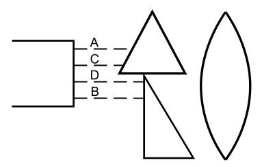
Aim four parallel rays into one face of the thinner of the two lenses of the kit as shown in the diagram below. Record the lens position, the ray paths and the focal point.
