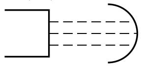
Record the incident and reflected rays and note where they meet. This point is called the FOCUS of the mirror.
