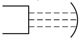
Move the Light Box sideways keeping the rays parallel to the axis of symmetry. Graph paper is useful to align the mirror and ray paths to ensure the rays are parallel to the axis.
