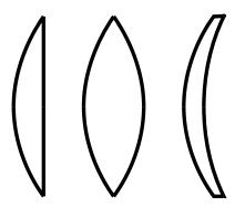
A lens may be the same shape as those in the kit, although many are shaped in a similar manner to those shown in the diagram above. The curvature on one side may not be the same on the other side and one side can be convex (bulging out) while the other side is concave (bulging inwards).
