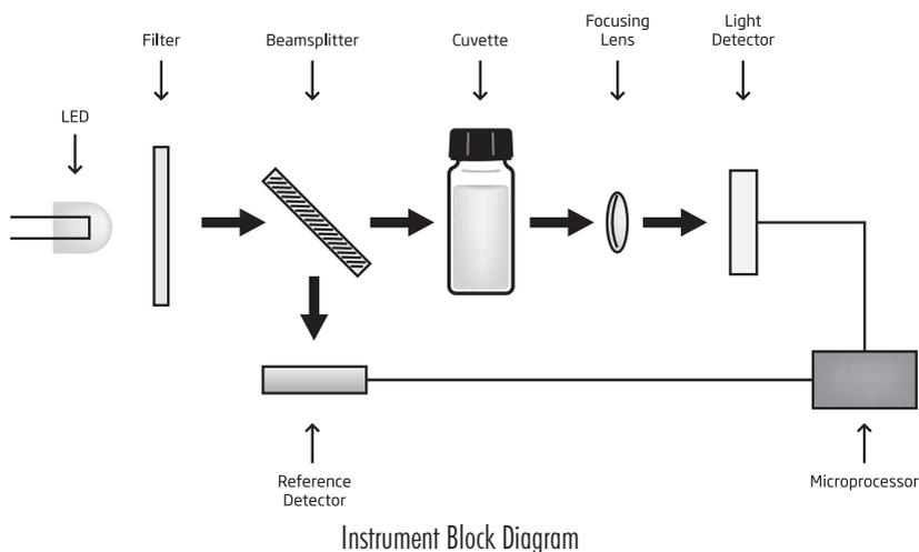
The internal reference system (reference detector) of the [HI83300](#) photometer compensates for any drifts due to power fluctuations or ambient temperature changes, providing a stable source of light for your blank (zero) measurement and sample measurement.
