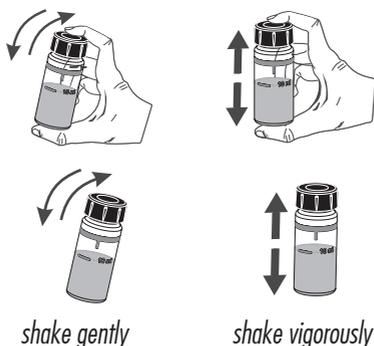
In order to avoid reagent leaking and to obtain more accurate measurements, close the cuvette first with the supplied HDPE plastic stopper
