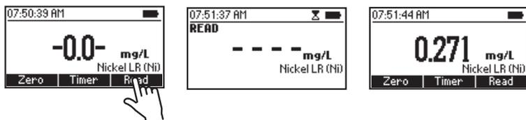
*Note: A temperature above 30 °C may cause turbidity. In this case add 2-3 drops of HI93703-51 Dispersing Agent to each cuvette and swirl until turbidity is removed before zeroing the meter and reading the sample.*
